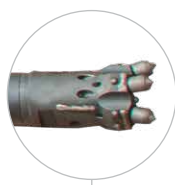
Rock drilling unit with roller chisel
