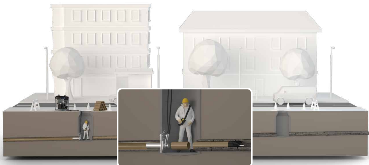
Application example: Renewal of a sewer pipe using the GRUNDOTIP pipe cylinder
